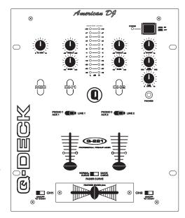
**CHANNEL TRIM LEVEL** - The channel trim levels are not to be used as volume controls, never use the channel trim to set the output volume. These controls are used to aid in distortion control. Use these control to preset your signal level before the crossfader. With your channel faders in the maximum position, use the channel trim level to set an average output level of about +4dB on you master level meter.
