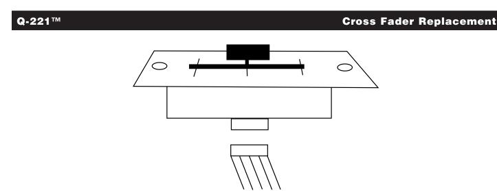
The crossfader is "Hot Swappable" which means it may be replaced at any time, even when power is applied. Only replace with American Audio Feather Fader Plus. Replacing with any other model fader may seriously damage your mixer.
