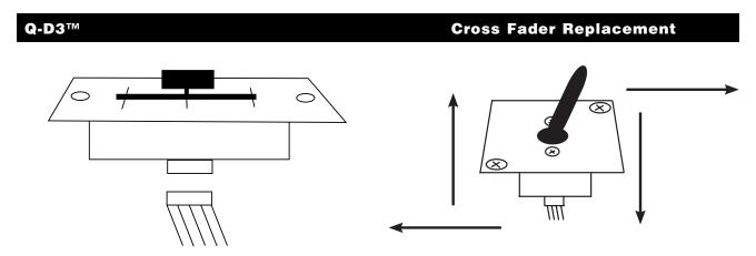
The crossfader is "Hot Swappable" which means it may be replaced at any time, even when power is applied. Only replace with American Audio Part Feather Fader Plus. Replacing with any other model fader may seriously damage your mixer.
