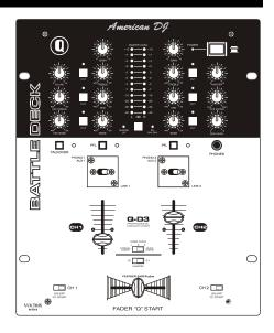
**CHANNEL TRIM LEVEL** - The channel trim levels are not to be used as volume controls, never use the channel trim to set the output volume. These controls are used to aid in distortion control. Use these control to preset your signal level before the crossfader. With your channel faders in the maximum position, use the channel trim level to set an average output level of about +4dB on you master level meter.
