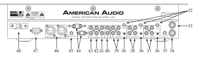
**32. GND (GROUND TERMINAL)** - Be sure to connect turntable ground leads to either or both of the two available ground terminals. This will reduce the humming and popping noises associated with magnetic phono cartridges.
