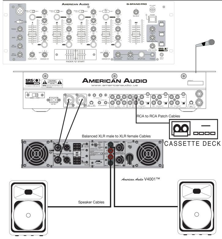
Typical Balanced Output Set-up
