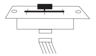
The crossfader is "Hot Swapable" which means it may be replaced at any time, even when power is applied. Only replace with American Audio Part Feather Fader Plus. Replacing with any other model fader may seriously damage your mixer.
