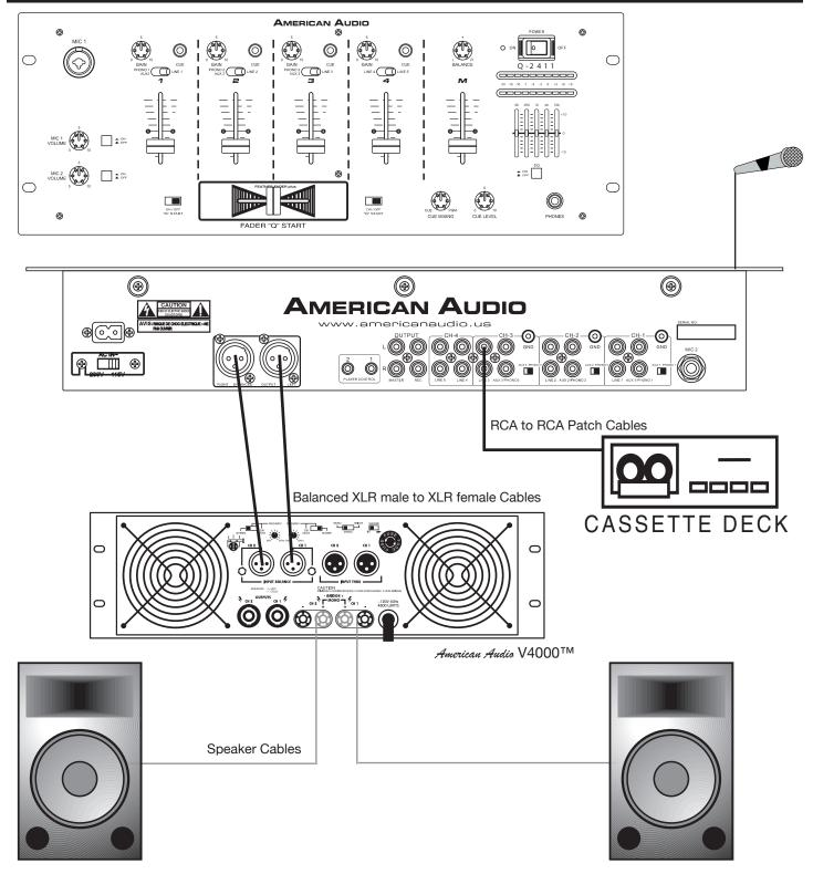
Typical Balanced Output Set-up
