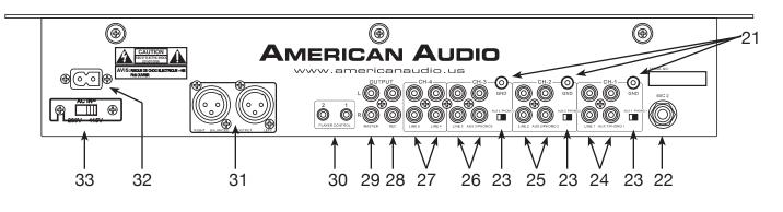
**21. GND (GROUND TERMINAL)** - Be sure to connect turntable ground leads to either or both of the two available ground terminals. This will reduce the humming and popping noises associated with magnetic phono cartridges.
