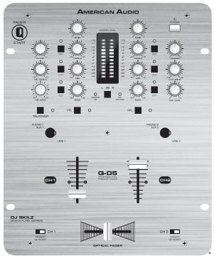
to set the output volume. These controls are used to aid in distortion control. Use these control to preset your signal level before the crossfader. With your channel faders in the maximum position, use the channel trim level to set an average output level of about +4dB on you master level meter.
