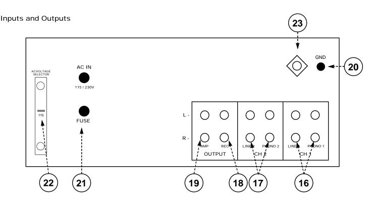
(16), (17) LINE / PHONO INPUT JACK - Input jacks for CH1, CH2, and CH3. Connect turntables equipped with MM pickup cartridges to the PHONO input. CD Players or Tape Decks should be connected to the LINE input. Line level musical instruments with stereo outputs such as Rhythm Machines or Samplers should also be connected to the LINE inputs.
