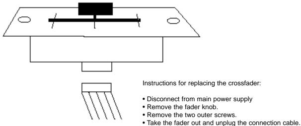
Connect the new fader and replace back into mixer.
