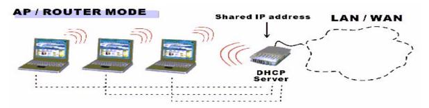
Figure 3. AP/Router Mode Configuration
