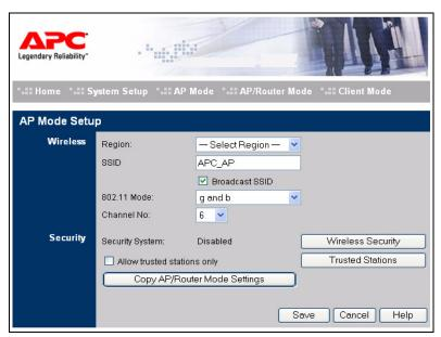
Figure 9. The AP Mode Setup Screen
