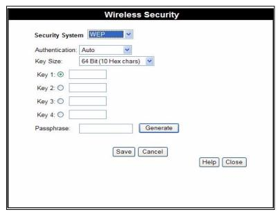
Figure 14. The Wireless Security Screen (AP Mode - WEP)
