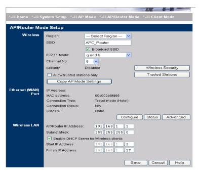
Figure 13. The AP/Router Setup Screen
