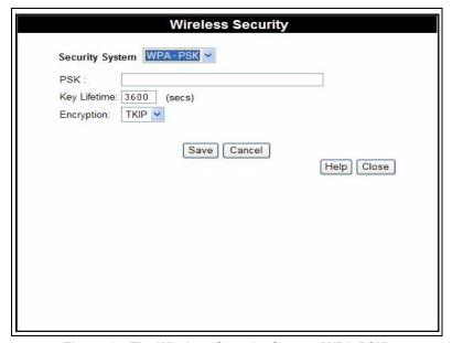
Figure 15. The Wireless Security Screen (WPA-PSK)
