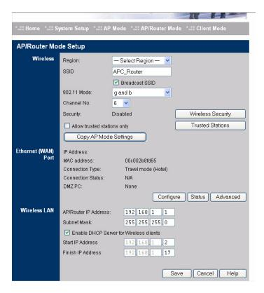
Figure 34. The AP/Router Setup Screen (annotated)
