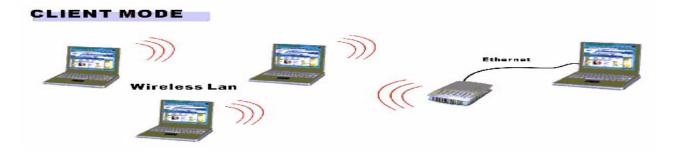
Figure 4. Client Mode Configuration
