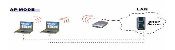
Figure 2. Access Point Mode Configuration
