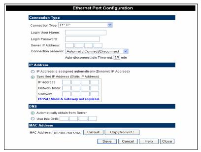
Figure 18. Ethernet Port Configuration (All Settings)
