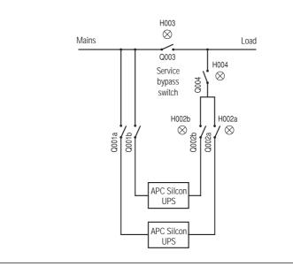
2.6.2 Switching the Parallel System from External Bypass into Normal UPS Operation
