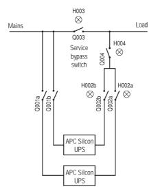
In a redundant system one UPS may be isolated for service/maintenance without affecting other parallel UPS(s).
