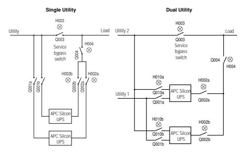
In a redundant system one UPS may be isolated for service/maintenance without affecting other parallel UPS(S).
