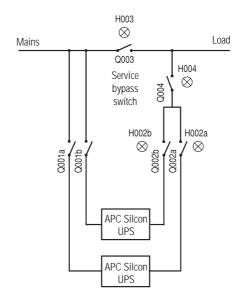
In a redundant system one UPS may be isolated for service/maintenance without affecting other parallel UPS(s).
