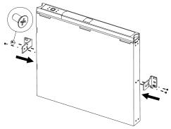
2 Note: Whenever possible, attach two screws into wall studs. If stud mounting is not possible, use an expandable wall anchor. Hardware is not included; .25" x 2" lag bolts are recommended. Mount the UPS in either of the displayed positions.
