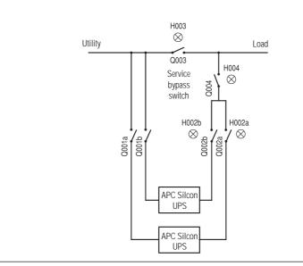
2.6.2 Switching the Parallel System from External Bypass into Normal UPS Operation
