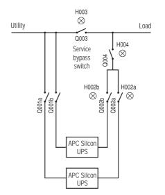
In a redundant system one UPS may be isolated for service/maintenance without affecting other parallel  $\mbox{UPS}(s).$
