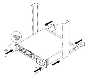
**5** Reinstall battery, battery bracket, and screws.
