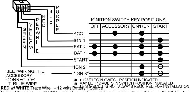
Connect this wire to a + 12 VDC constant source found at the vehicle's ignition switch using the 30 Amp fuse and holder provided. This wire provides power for the control circuit as well as the ignition 1 and ignition 2 relays.
