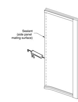
Tub Surround Adhesive (studs) Sealant (tub edge)
