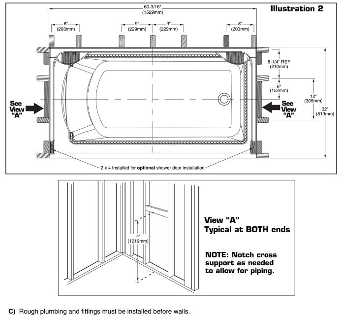
NOTE: <u>Installation over greenboard or firewalls</u>: If installing wall panels over greenboard and/or firewall material, and not directly on the studs, your alcove dimensions must consider the thickness of this material. Measure from the inside of the finished walls.
