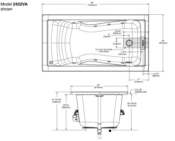
DIMENSIONS OF FIXTURES ARE NOMINAL AND MAY VARY WITHIN THE RANGE OF TOLERANCES ESTABLISHED BY ANSI STANDARDS Z124.1 AND A112.19.7.
