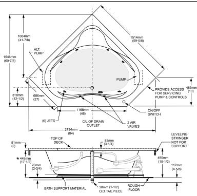
\* NOTE: If the optional apron (PN 0730.121) is to be used with this tub, the stringer height must be referenced from the finished floor.
