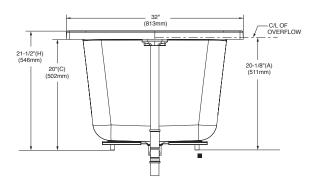
DIMENSIONS OF FIXTURES ARE NOMINAL AND MAY VARY WITHIN THE RANGE OF TOLERANCES ESTABLISHED BY ANSLSTANDARDS 7124 1 AND A112 19 7
