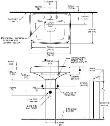
▼ DIMENSIONS SHOWN FOR LOCATION OF SUPPLIES AND "P" TRAP ARE SUGGESTED. ▼ PEDESTAL ANCHORING SODE WEAK
