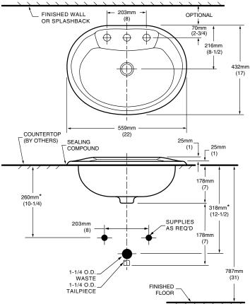
${\bf NOTES:}$  \* DIMENSIONS SHOWN FOR LOCATION OF SUPPLIES AND "P" TRAP ARE FOR COUNTERTOP CUTOUT AND INSTALLATION INSTRUCTIONS USE TEMPLATE SUPPLIED WITH SINK.
