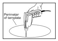
Cut opening around the perimeter of the template.
