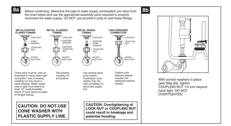
**WARNING:** Do not use plumber's putty, pipe dope, or any other sealant on the water supply connection to this tank. If the connection leaks after hand tightening, replace the supply line. If the connection continues to leak with the new supply line, replace the fill valve. **Warranty is void if any type of sealant is used on the water supply connection.**
