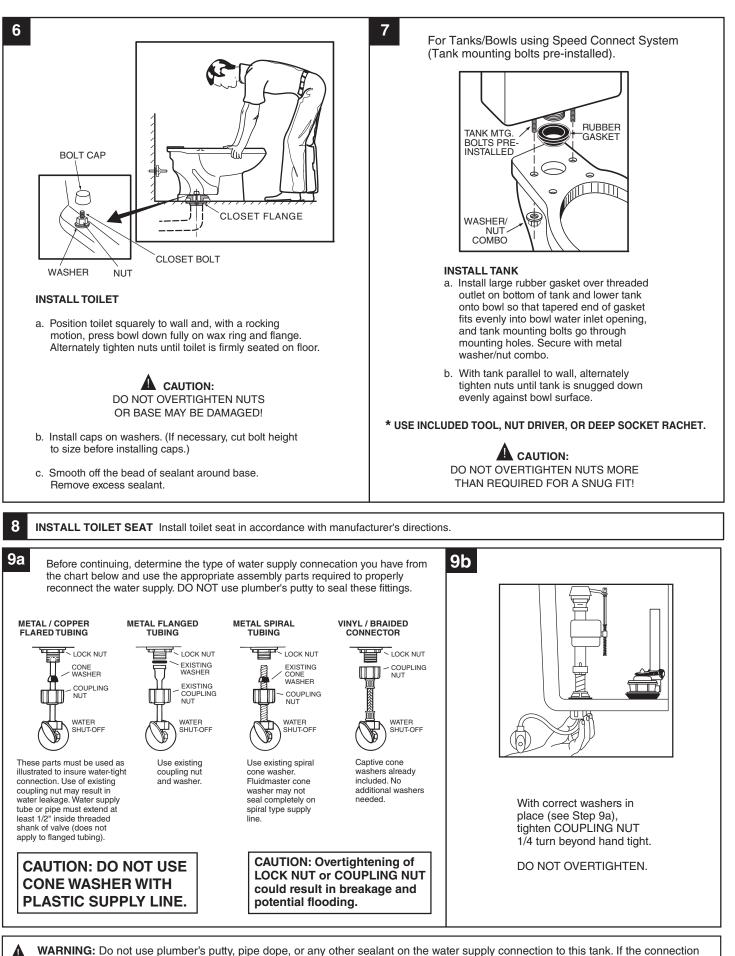
WARNING: Do not use plumber's putty, pipe dope, or any other sealant on the water supply connection to this tank. If the connection leaks after hand tightening, replace the supply line. If the connection continues to leak with the new supply line, replace the fill valve. Warranty is void if any type of sealant is used on the water supply connection.
