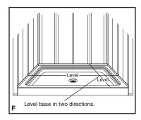
**Note:** Allow the bedding material to completely harden before applying weight to the bottom of the shower base.
