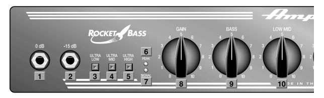
**1. 0dB Input** accepts a standard 1/4" instrument plug from your bass. This input is suited for use with instruments that have passive electronics.
