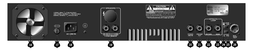
**16. FAN:** This temperature controlled, variable speed fan draws cool air into the amplifier, forcing heat out through the exhaust vents (also on the rear panel, between the speaker jacks and the power amp in jack). Never block the vent holes or the fan openings.
