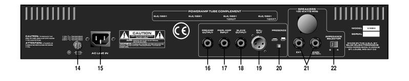
**14. FUSE:** This protects the unit from damage due to overload conditions or power line surges. If the fuse blows, replace it only with the same size and type.
