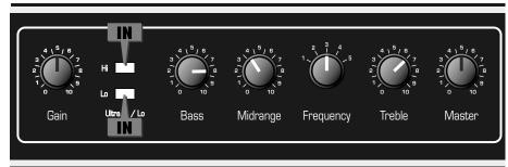
The Master should be set to produce the appropriate output volume level.
