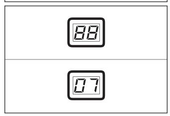
**4.** After a slight pause, the pump will start and the system pressure will be displayed. This number will increase as the pump runs and the tank fills.
