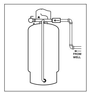
**5.** Plumb the outgoing supply to the building's water supply system or into the water treatment equipment (if present).
