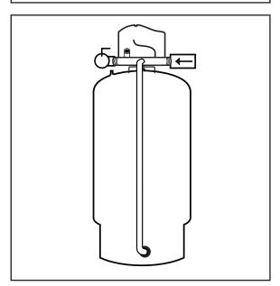
**4.** Connect the water line from the well pump to the inlet of the Well- $X1^{\mathsf{TM}}$ .
