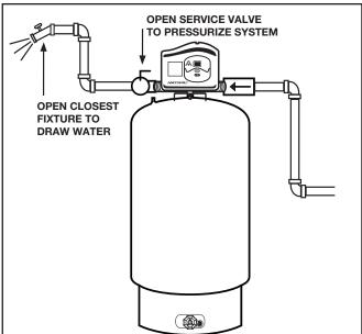
7. When the system reaches the factory cut-in (pump on) setting of 40 psig, the pump will start. Like a traditional mechanical switch, the pressure will begin to rise, repeating the cycle. If desired, the Well-X1™ settings can now be adjusted as shown below.
