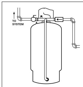
**6.** Install a blow down tube from the relief valve to a drain or to within 6" of the floor as required by local codes.
