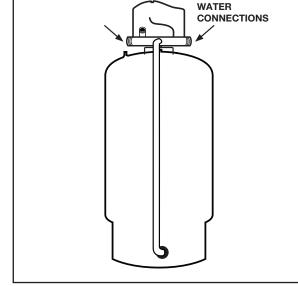
**2.** Install the supply piping from the well pump. If required, install a spring-loaded check valve.
