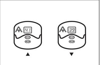
3. To adjust the cut-out, depress **MODE** once and the display will read **HI**. Again, press the **V**or ▲ buttons to raise or lower the setting. The same 10-55 psig differential range applies.
