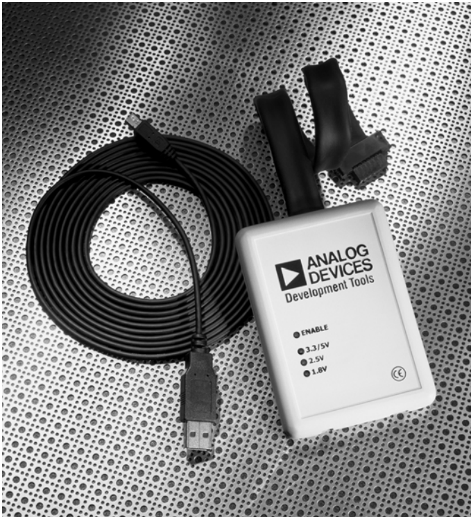
Figure 2-18. High Performance USB 2.0 JTAG Emulator
