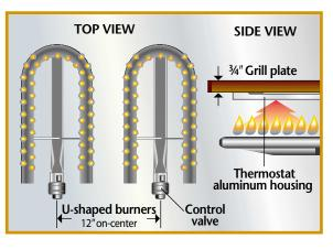
The U-shaped burner design covers more surface area than conventional straight burners. Heat is more evenly and widely distributed under the grill plate, allowing you to maximize the use of the grill surface for better consistency and productivity.
