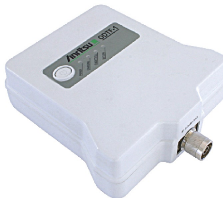
Using a VNA Master equipped with Option 0002 or 0501, this ODTF-1 optical module translates the optical signals to the RF domain of the VNA, to display fault locations in standard optical fibers.
