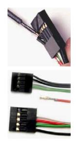
3. Working carefully so as not to damage the wires, connectors or pins, slowly reinsert the pin into the correct slot of the connector then snap closed the black tab that was lifted in step 1. Repeat these steps for each wire you need to change.
