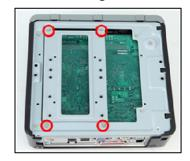
3. Attach the red insulating strips by removing the adhesive covering and attaching them as shown in the picture.
