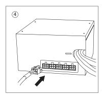
Connect the AC power cord to the power supply AC inlet and turn the switch to "I" position.
