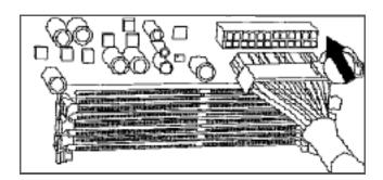
3. Connect the 8-pin or 4-pin ATX12V connector for the CPU to the appropriate connector on your motherboard. If your motherboard has an 8-pin socket with a cover on some of the openings, we recommend that you remove the cover and use the 8-pin connector.
