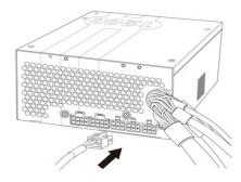
5. Connect the AC power cord to the power supply AC inlet. Please be sure to use the heavy-duty cord supplied with your TPQ-1200.
