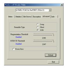
There are **Preamble Type**, **Fragmentation Threshold**, and **RTS/CTS Threshold** setting under this mode.
