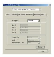
Additional security can be achieved by using the WEP (Wired Equivalent Privacy) encryption. WEP encrypts each frame transmitted from the radio, using one of the keys entered from this panel.
