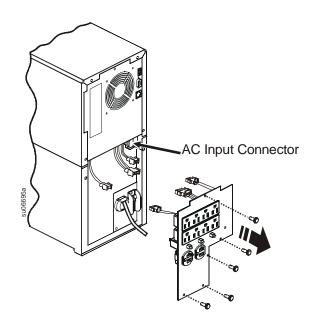
Locate and snap together the corresponding connectors on the UPS and the replacement PDU panel.
