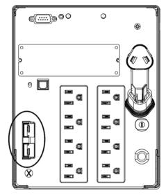
This figure shows the location of the battery pack connector.
