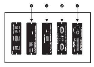
**Daisy chains** If you have increased your SmartSlot capacity by daisychaining Expansion Chassis or Triple Chassis, install the PowerNet SNMP Adapter (or Web/SNMP Management Card) and Call-UPS*II* in the highest-numbered and secondhighest-numbered slots, respectively, of the chassis installed farthest from the UPS.
