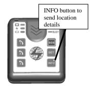
□ The device will collect GPS data (ca. 30-60 sec) and send a message and GPS coordinates to the Control Base. The Control Base software will find the street name and closest intersection from a map server and send these details through SMS short messages to all Contact numbers, with the text (*example*):
