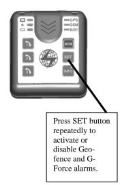
□ If a Geo-fence alarm has been triggered, the device will send an alarm message and GPS coordinates to the Control Base. The
