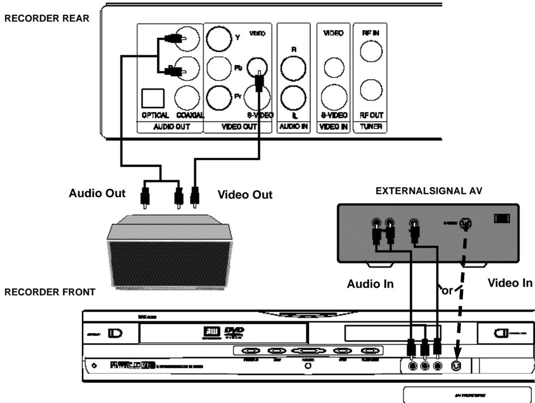
Connect your recorder with the S-Video cable, if the Signal Source has an S-Video input. Do not connect the yellow video cable if using the S-Video cable.
