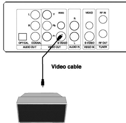
Connect your recorder with the S-Video cable, if the TV has an S-Video input. Do not connect the yellow video cable if using the S-Video cable.
