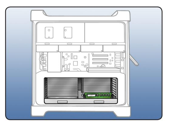
2 Press down and release 2 latches on front of processor tray.
