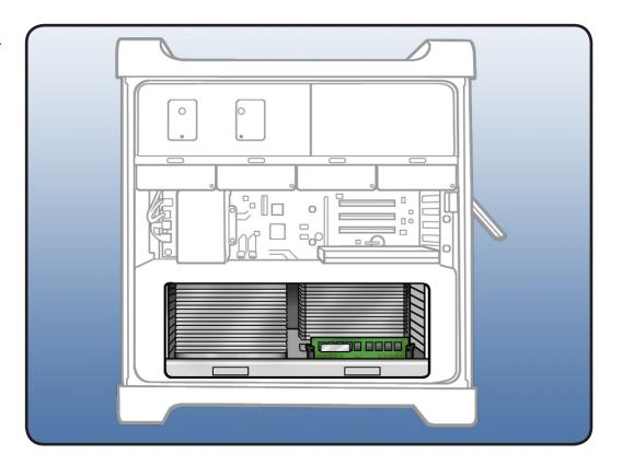
**11** Press down and release **2** latches on front of processor tray.
