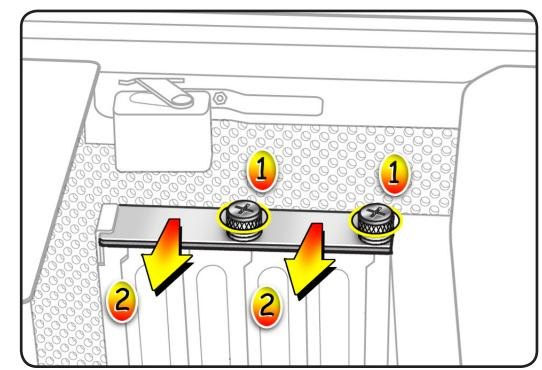
**Note:** Card is held in place by retention bar. Following two steps explain how to release bar.
