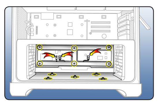
**Note:** Processor cage includes two fans, one at each end of cage. Before removing cage from enclosure, you must release 2 latches on each fan and push fans partway into cage.
