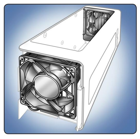
2 Release fan cables from clips on bottom of processor cage.
