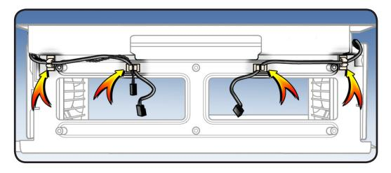
**3** Release **4** latches on front fan and slide fan out of cage.
