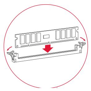
10 Align the notches on the memory module with the small notches inside the slot. Push down the DIMM until it snaps into place.
