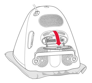
6 Touch the metal shield that is visible inside the recessed latch area before touching any components on the main logic board. This helps protect the computer from damage caused by electostatic discharge.
