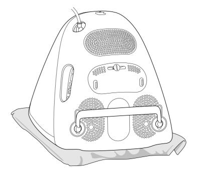
4 Use a coin or screwdriver to turn the latch on the access door.
