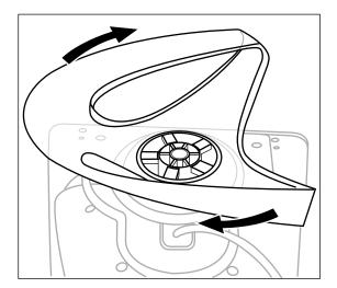
7. Peer into the center of the monitor stand and swivel it somewhat until you can see the locking tabs line up with the slots in the base.
