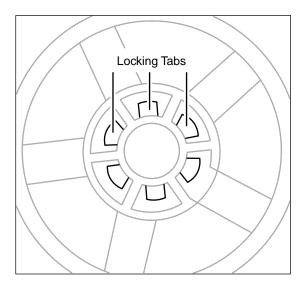
8. With the tabs aligned, gently pull the stand toward you. Then tilt the stand up off the base.
