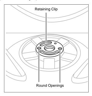
Using two jeweler's flat-blade screwdrivers, place one in each of the round openings and gently pry up the retaining clip until it is out of the monitor stand.
