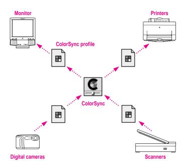
ColorSync performs color matching by comparing each profile to an independent color standard. ColorSync uses the CIE color standard, which describes colors in terms of how they are perceived by the human eye under specific lighting conditions. (CIE stands for the Commission International de l'Eclairage, the International Commission on Illumination, which created the standard in 1931.)
