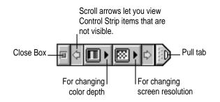
The Control Strip is a quick and easy way to make changes to the features you use most on your computer, such as screen resolution and color depth.
