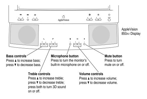
Bass, treble, and volume adjustments have an onscreen indicator that appears when you press a button on the front of the monitor. For example, pressing the Bass button displays the Bass indicator.
