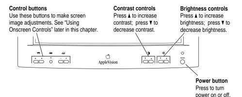
The contrast and brightness adjustments have an onscreen indicator that appears when you press the contrast and brightness control buttons on the front of your monitor. When you make an adjustment, the indicator bar moves to show the current setting. When you've finished making adjustments, the indicator disappears automatically.
