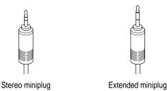
If your equipment has a different type of connector, you can purchase an adapter at an electronics supply store.
