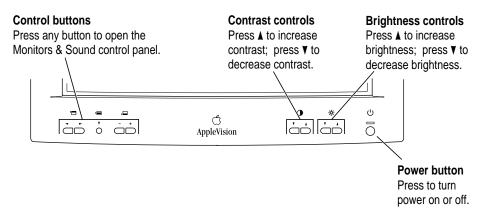
The Contrast and Brightness adjustments have an onscreen indicator that appears when you press a button on the front of your monitor. For example, pressing a Brightness button displays the Brightness indicator.
