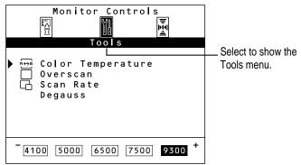
Use the Tools menu to set color temperature, turn overscan on and off, display the scan rate of your monitor, manually degauss, and turn speakers on or off in sleep mode.
