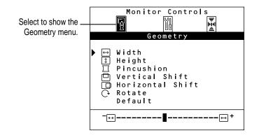
Use the Geometry menu to adjust the height and width of the screen image, center the image on the screen, and so on.
