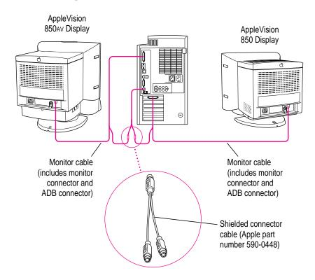
**IMPORTANT** Make sure you use an Apple *shielded* connector cable. Most thirdparty ADB splitter cables are not shielded and will not work properly with your AppleVision monitor. (You may experience more radio interference with an unshielded connector cable.)
