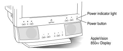
If you plug your monitor directly into your computer, no power indicator light goes on until you start up your computer. If you plug your monitor into a wall outlet, the monitor's amber power indicator light goes on. When you start up your computer, the indicator light turns green.
