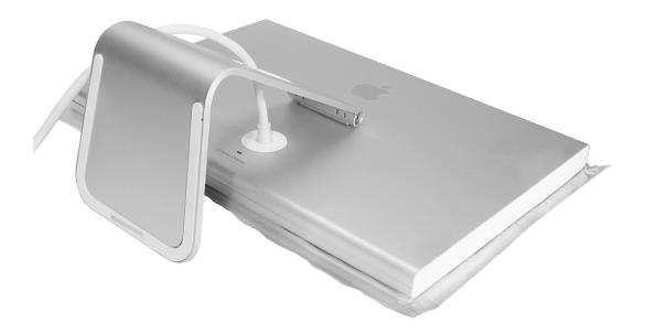
2. Copy the serial number from the old stand to the blank serial number label. Affix the label to the same area on the replacement stand.
