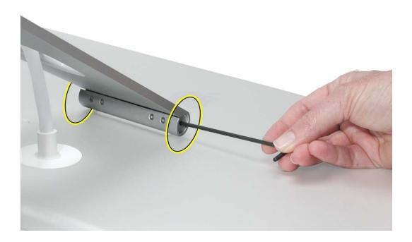
4. With the screws removed, grasp the stand, and pull it off of the mounting bracket.
