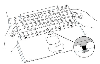
3 Pull down on the keyboard release tabs (located to the left of the F1 and F9 keys) and then press down on the top portion of the keyboard.
