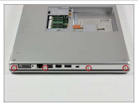
Remove the four 3.2 mm Phillips screws on the port side of the computer.
