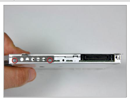
Remove the two Phillips screws securing the mounting bracket to the rear of the optical drive.
