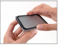
• For 7 mm SSDs, you'll need to apply a spacer to ensure a good fit.
